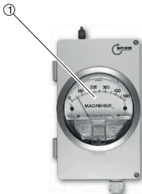
Fig. 11: Analogue differential pressure gauge
