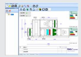
Example of selecting a EUROVENT-certified TKM 50 N EU unit fitted with a rotary recovery system.
