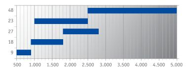
TBS-EC: Air volume flow range depending on model. Q in m<sup>3</sup>/h.
