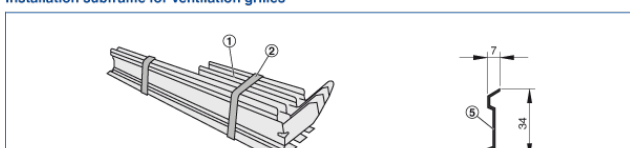
Installation subframe for ventilation grilles
