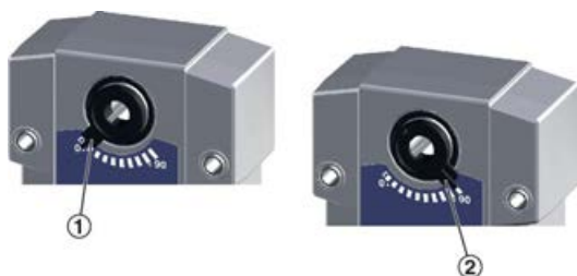
Fig. 51: damper blade position indicator
