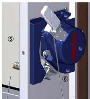
Fig. 48: Close the damper blade
