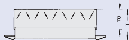
... - AG Opposed blade action volume control damper, adjustable from the front face.
