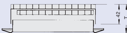
... - AS, -KS, -RS Volume control of hit and miss construction with stamped vertical blades, adjustable from the front face.
