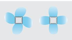
Individually adjustable discharge direction with the optional air control blades
